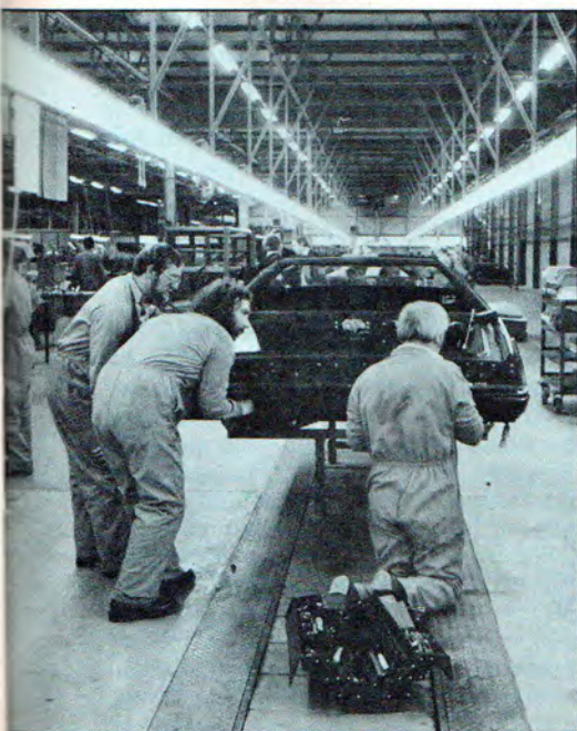
Assembly line in De Lorean plant is designed to keep workers from having to make overhead reaches.
